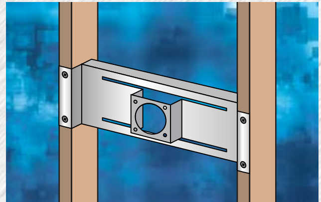
figure 1. SolidDrive SD1 mounting bracket attached to wall studs.
